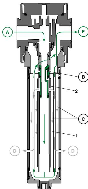
A. Compressed air enters the body of the dryer and, through the pipe located at the center of the membrane (1), flows downwards. At the bottom, the flow direction is inverted, and the air rises, passing through the membrane.
