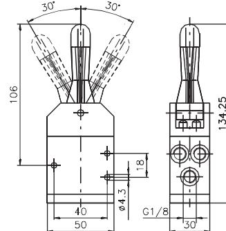
Lever central Metal (spring 3 pos.) One position stable
