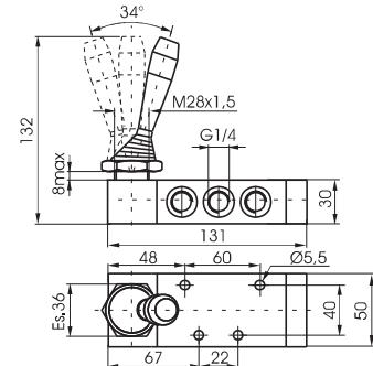
► **Lever lateral with locking device - 2 positions**
