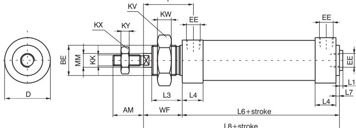
Version derived from standard execution 1260 and not included in ISO standard. Not having a rear eye it is shorter and the air inlet is from the rear or at 90° like it is on the front. The considerations made for the basic type 1260 apply for all single-acting types.
