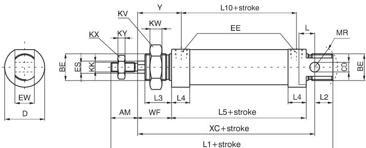
Similar overall dimensions as 1260 basic type, it differs because of the hexagonal rod (instead of circular) to avoid the rotation. It is particularly suitable when it is used as a guide and support to the linked element. Not for use with high frequencies and long strokes. For which, whenever possible use front spring.
