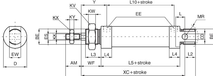
Standard execution, fully complying with ISO standards from Ø8 to Ø25. Bores 32, 40 and 50 not included in the standard, comply with our own specifications. Can use all available mountings. For single acting type, the maximum stroke is 40 mm., after which overall dimensions increase in length to an extent not proportional to the stroke (and in any case not longer than stroke 100).
