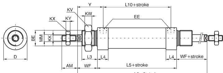
Execution by rod coming out from both end caps, with overall dimensions, except for the rod, equal to 1260 version. Not available with Ø8 and 10.
