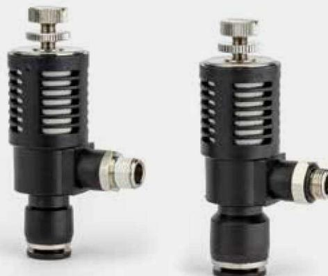
The quick exhaust valve always used to the shuttle valve and cylinder, the air can be exhausted quickly and not through the shuttle valve, which fast the reciprocating motion on the cylinder and short the work period. The exhaust side T have the function with throttling and noise elimination. It can control the high-speed cylinder, at the same time also can reduce the exhaust noise.
